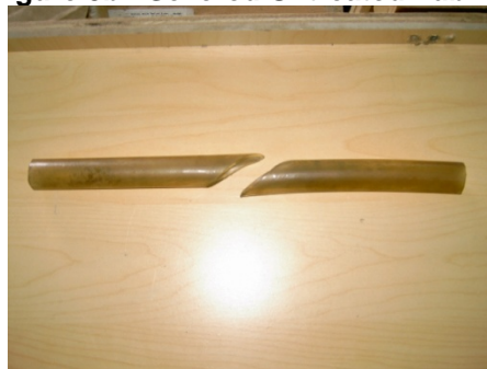
Figure 3b: Severed Untreated Tubing
